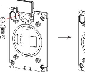
2A. Place the device (not included) into the bracket from above as illustrated. Use provided screws (C) and rotate in from below with screwdriver(not provide) until securely fastened.
