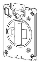
1A. Align bracket (A) with the compatible case (not provided). Using the provided tool (D) rotate in (4) screws (B) through the aligned holes of the bracket and case until securely fastened.
