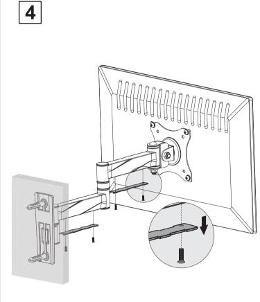
Step 7: For cable management, unscrew two provide plates to the bottom on the mount arms.
