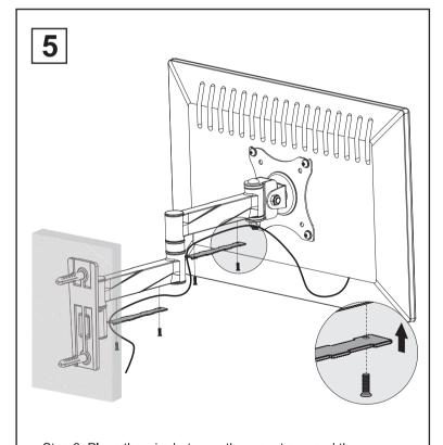
Step 8: Place the wire between the mount arm and the plate, and secure screws again so cables remains in place.
