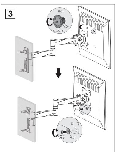
Step 6: To attach monitor, or other VESA compatible device with threads, insert screws through the back of the mounting plate and into the device to achieve secure and sturdy placements.
