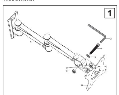
STEP 1: Place two washers, " part D" inside of the U-Shape Connector on the back of the VESA plate.
