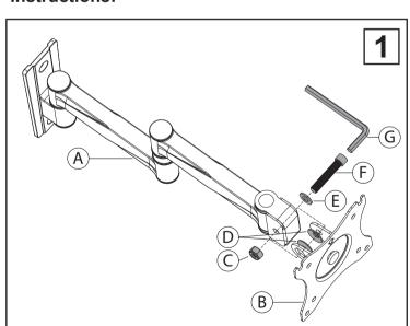
STEP 1: Place two washers, " part D" inside of the U-Shape Connector on the back of the VESA plate.
