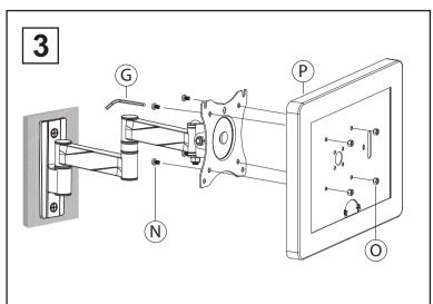
Step 6: To attach enclosure "P", insert screws "N" through the back of the mounting plate while holding the nuts "O" from the front, then rotate using included allen key tool "G" until securely tightened.
