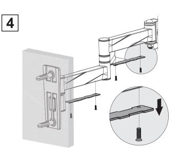
Step 7: For cable management, unscrew two provide plates to the bottom on the mount arms.
