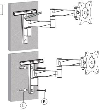
Step 4: To drill to the wall, use pencil to mark your aim points on the surface.
