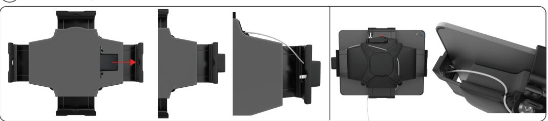
**LEFT:** Take the rubber security component, line it up with the holder arm that you wish to slide into. The component should line up to the cords that gets plugged into the tablet With the holder arms extended, place the tablet into the center with the cord plugged in. Arrange and wrap the power cord of the tablet into the rubber security component. Push inwards all arms of the holder until you have a secured and tight fit.
