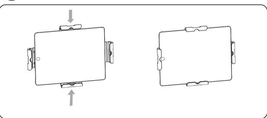
While holder is in 'unlocked' mode, extend the arms outwards until tablet fits comfortable in place. Retract arms until they hold the tablet firmly. Tablet holder can accommodate tablets in cases as well up to 1" thick.
