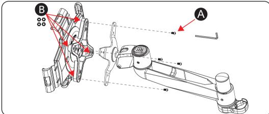
Line up the VESA plate of PAD-VTH to the correlating VESA to be affixed to. On the same side of the PAD-VTH VESA, place the hexagon nut in the screw hole groove. It will be semi-recessed when nut is placed. (Letter B) While holding the nut with one hand, and from the side opposite of PAD-VTH (shown above with letter A), use the included allen key and screw in bolts into the hole until tightly secured.
