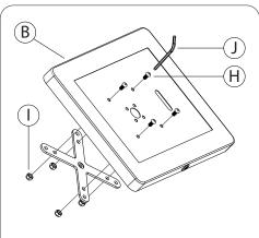
2A. Screw in the (4) screws (H) from the front through the enclosure and VESA, while holding the hex nuts (I) from behind using the allen key tool (J) until securely tightened.
