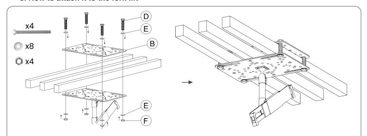
3A. First, take the two metal rectangular plates (B) and sandwich the forklift roof bars as illustrated and insert bolts, washers and nuts (D, Ĕ, F) rotate them until securely tightened.
