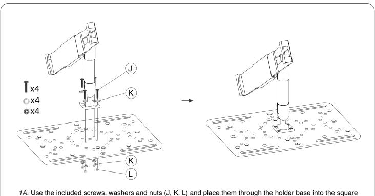
1A. Use the included screws, washers and nuts (J, K, L) and place them through the holder base into the square metal plate (B) holes, screw it in with a screw driver while holding the nuts from behind with your fingers until securely tightened.
