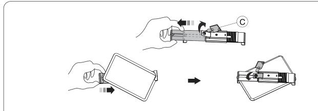
2A. Insert key (C) into lock at back of holder. Turn counterclockwise to unlock, then slide to open. Insert tablet against fixed end, then slide down to hold tight. Turn key clockwise to lock.
