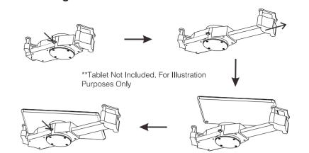
3A. Press the release button on the side of the holder. While holding the button, extend the arms so you're able to insert your device. Press the button again to retract arms and firmly grip at the corners of your device securely
