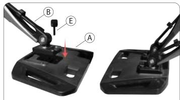
2A. Slide the articulating arm into the dedicated mount location on the base. Rotate in screw until moderately tightened with your hand, no extra tools needed. Repeat to the other side.
