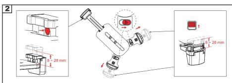
How to install the base on the wall: (A.B.C.D.E)
