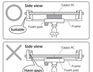
Paste method Backing 1. Tear off the backing paper paper on the foam pad. 2. Stick the foam pad to the frame as shown in the right picture. Align the holes Adhesive side
