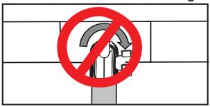
DO NOT attempt to adjust, tilt, or rotate any ball socket joints while it is fully tightened. Any such action will result in possible damage and loss of integrity of product functioning at full capacity. Manufacturer will not be responsible for any such actions by any person.
