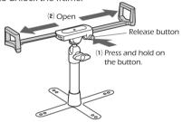
2. Install the tablet PC on the frame.
