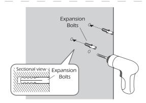
1. Drill a hole in the wall to these specifications: diameter: 6.5~7mm; depth: 40~45mm Knock the expansion bolts completely into the wall.
