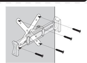
2. Fix it with screws on the wall.
