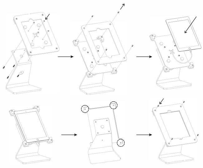
4 Fitting corners are pre-installed. If position not accurate when install tablet, first loose the corner screws a little and adjust the corner position to fit the tablet. Tighten again after adjustment.
