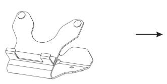
3. Pull back the sticker and adhese the anchor onto the desired surface and the lock adhesive on the back of the tablet. Make sure to have the loop of the cable on the anchor before adhesing it to the surface.
