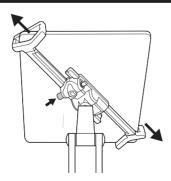
2. Press and hold on the release button to unlock the frame.
