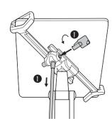
1. Insert the key into the lock button to release the cable.
