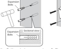
1. Drill a hole on the wall. 2. Knock the expansion 3. Fix it with screws bolts completely into on the wall. the wall.
