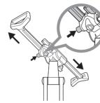
1. Press and hold on the release button to unlock the frame.
