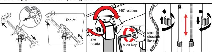
1. Press and hold on the release button to unlock the holder,place tablet against corner then slide in
