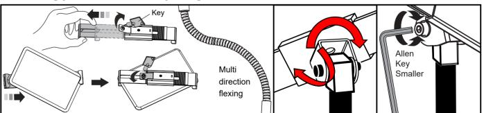
unlock, then slide to open. Insert tablet against fixed end, then slide down to hold tight. Turn key clockwise to tighten.
