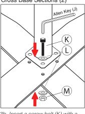
3b. Insert a screw bolt (K) with a washer (L) into each of 4 holes. Place another washer (L) on the underside of each screw bolt. Grip the nut (M) on the underside with one hand, and use the other tighten each screw with the allen key tool (J). Repeat for all four screw bolts.
