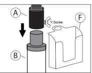
4a. Place battery case (F) over top of metal connection. Note: if the Y screw is already in, unscrew before attaching the gooseneck.
