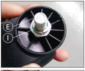
2a. Place a spring washer (I) over the screw bolt on each caster (E).
