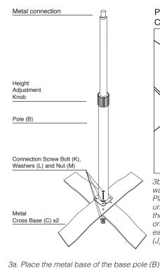
Pole Assembly and Pole Nut Cross Base Sections (2)
