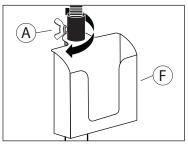
4b. Screw the gooseneck onto the metal connection of the pole by turning clockwise. Be sure that the battery case is on the opposite side of the pole as the Y screw.
