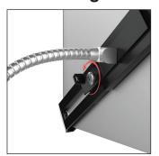
5a. Insert key (O) and set position to unlock. Remove key, then slide holder (A) open.
