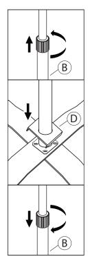
3c. Rotate the grip counter clockwise to loosen completely and remove from the top of the pole.
