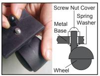
Place the screw bolt from each wheel through the metal base, then place a nut cover over the top of each. Screw down clockwise by hand, then use wrench to tighten further.
