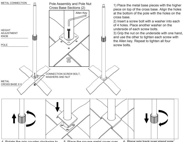
4. Rotate the grip counter clockwise to loosen completely and remove from top of pole.
