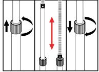
3. Rotate plastic grip counter clockwise to loosen, then adjust pole to desired height. Rotate plastic grip clockwise to tighten.
