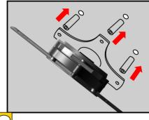
Insert the plastic insert into the hole align the holes on both "X" metal plate and the wall.
