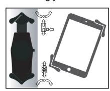
Press button on side of tablet holder to slide open.Insert your tablet against spring arm,then slide other end back down.
