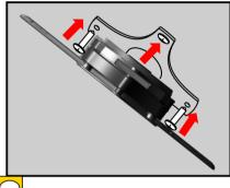
crew up the screws one by one to connect the Wall Mount to the Wall.
