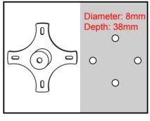
1. Make 4 holes on the wall according to the holes position on the "X" Metal Plate of the Wall Mount.
