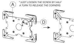
3A: Begin inserting your tablet device into the holder by loosening the holder corner arms. Find the screw on the body (A) as illustrated and loosen all (4) with provided special allen key tool (D).
