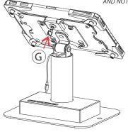
4A: Take the keys (G) and insert into security lock and rotate. If a button pops out, when you remove the key, then you know the holder is in unlocked position. To lock the holder, you simply press down the security button until it clicks and then you'll know it's locked.
