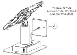
7A: Identify the charging hub at the base. Make sure to use plug in a charging plug into the Type-C charging port in order for your tablet to charge properly. Also double check that the wire above is plugged in
