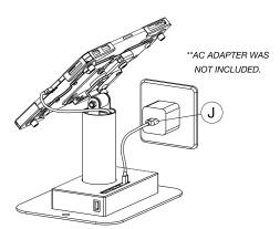
7B: You also can charge with an AC adapter(not included) on the wall outlet.
