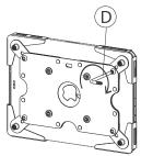
3D: While all the arms are tightly and secured on the tablet edge corners, go back to the backside and using special allen key tool (D) rotate the opposite direction for all (4) screws until securely tightened.
