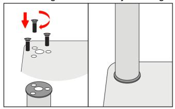
1. Align the pole and plate using the three holes. Screw them together from the bottom up using included screws.
