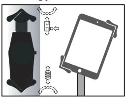
Press button on side of tablet holder to slide open. Insert your tablet against spring arm. Slide other end back to secure device.
