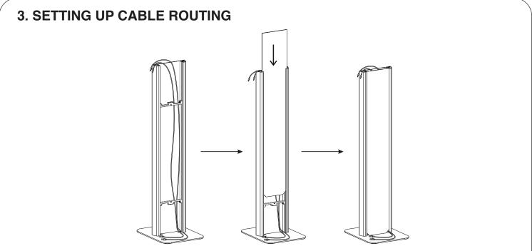
WITH ONLY (1) PANEL BACK IN, SLIDE IN THE POWER CORDS AND ANY OTHER CORDS THAT WOULD NEED TO BE CONNECTED TO THE TABLET THROUGH THE BODY AS SHOWN. THERE WILL BE GAPS AT THE TOP AND BOTTOM FOR THEM TO ROUTE OUT TO THE POWER SOURCE AND TO THE DEVICE. SLIDE IN SECOND PANEL WHEN ROUTING IS FINISHED.
