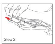
Peel away plastic frame starting with the bottom of the case as shown to the left. Work your way around the perimeter, unclipping the frame where there are clips.
