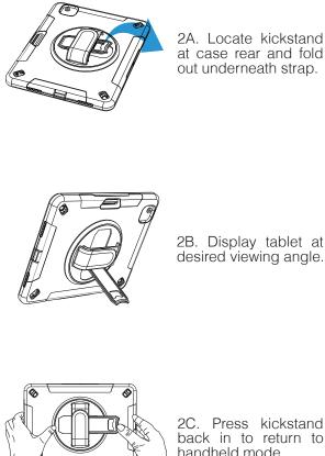
2A. Locate kickstand at case rear and fold out underneath strap.
