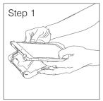
Starting at a corner of the case, peel away the sillicone jacket. Work your way around until only the hard case remains.
