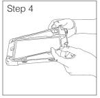
Re-insert the front frame back on. Make sure you go around the perimeter of the case and clip all the clips securely and tight.
