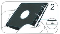
Gently apply pressure to the small clips (as indicated by the arrows) and unclip all four sides. Once all the sides are unclipped, the internal hard case will open.
