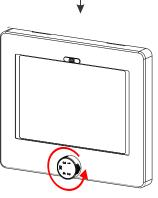
9B. After, turn the digital lock 90 degrees clockwise. This will lock the tablet in place.
