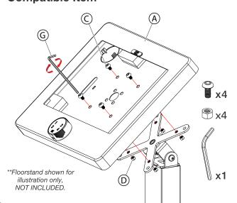
7A. Align enclosure holes to VESA plate holes. Screw in the screws (C) above using provide allen key (G) while holding hex nut tool (D) from behind with fingers.
