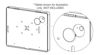
6A. When installing device into the enclosure, identify where the camera is. Then simply remove and pop out the cover prior to mounting or setting up tablet to properly expose camera.
