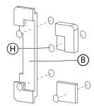
3A. Identify the double sided adhesives (H). Peel away the backing on both sides. Adhesive four of them behind the foam pieces (B) as illustrated. They are to adhese the foam to the enclosure. Peel away the back on the next four and place them on top of the foam pieces as illustrated. These are to attach the foam to the tablets and ensure security.
