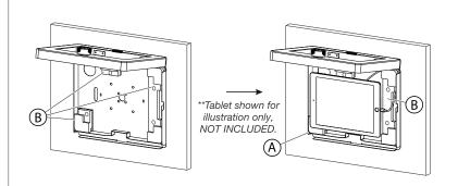
4A. With the enclosure open, insert tablet into the foam adapters (B). Make sure the adhesives have been placed ahead of time or tablet will fall out. Plug your tablet into any cables/wires you have routed to the enclosure. After tablet is secure, close the top and lock into place.
