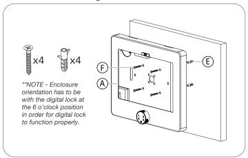
1A. Align the enclosure to the wall and mark off the holes with a pencil (not included). Use a drill (not included) and predrill locations. Insert (4) anchors (E) as illustrated into the wall drilled holes. Then align VESA holes of enclosure and rotate in screws(F) until securely fastened.
