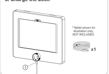
8A. Identify the lock chart port on the bottom side as illustrated. Plug in provided charging cable from one end to another to properly charge digital lock.
