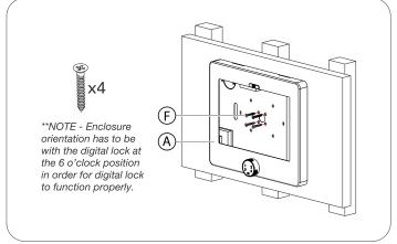
2A. Identify the wall studs behind the wall. Align the inner VESA holes as illustrated. Then using a screwdriver(not included), rotate in the (4) screws(F) until securely fastened.
