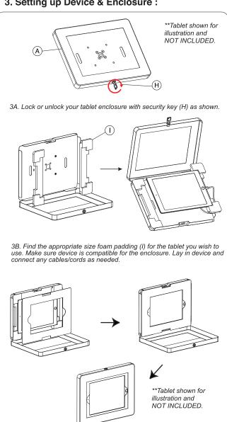
3C. If needed, lay-in correct included masking insert (I). Close and lock enclosure afterwards and you're set
