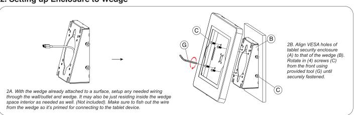
3A. Align enclosure holes (A) to VESA wedge holes (B) then turn in screws (C) using provided tool (G)
