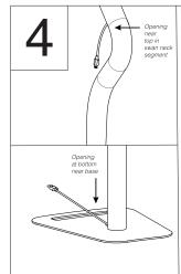
STEP 4: (Optional) Assembly core has a product design for cable management. Insert cables/power cords through opening at the bottom and extend through the body all the way to the opening at the swan neck segment to attach cord to tablet.
