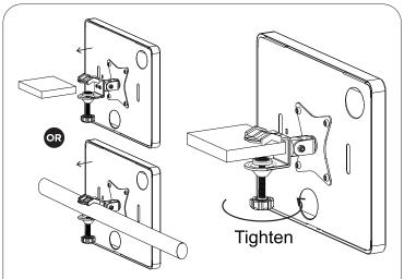
2A. Insert the surface between the clamp piece (B). Then, tighten the clamp by rotating the knob clockwise.
