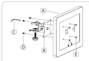
1A. Align enclosure (A) holes to VESA plate (B) holes. Rotate in screws (D) from behind using the provided allen key tool (C) while holding the hex nuts (D) from behind as shown above.
