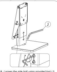
2A. Loosen the side bolt using provided tool (J) to raise or lower to height to your preference. Rotate opposite direction to securely tighten and set your height.
