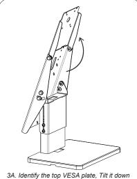
for a 2-direction setup or keep it up for a 1-direction setup as required.
