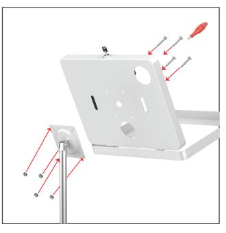
Combine nuts and bolts through VESA plate from the front & back as shown with provided tools.
