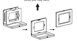
4 - If needed, make sure to lay-in the correct masking cover. Then close and lock the enclosure and you're ready to go.
