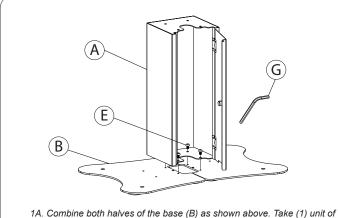
1A. Combine both halves of the base (B) as shown above. Take (1) unit of the body (A) and align the mounting holes. Rotate in (4) screws (E) with provided allen key until securely tightened.
