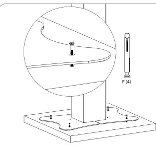
4A. Drill (4) holes into the surface using a power drill or like (not provided). Take the metal anchor (F) and place the casing into the holes. Then take the screw end and rotate in with screwdriver (not included) until securely tightened.
