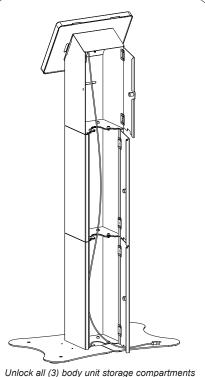
Unlock all (3) body unit storage compartments using the correct key for each section. Fish the cables through as shown and out the opening at the very bottom as needed.
