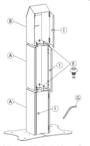
3A. Find the other body unit (A) and the printer shelf component. First unlock the compartments using the keys (I). Then align holes between two body units at a time. Take (4) screws (E) and using the provided allen key tool (G), rotate in the screws as shown until securely tightened.
