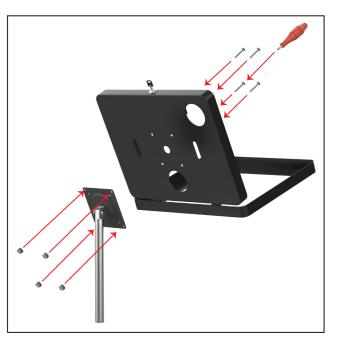
Combine nuts and bolts through VESA plate from the front & back as shown with provided tools.
