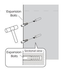
2. Knock the expansion bolts completely into the wall.
