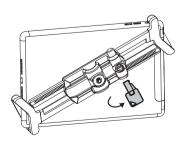
1. Insert the key into the lock slot to unlock the frame.
