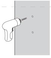
1. Drill a hole in the wall to these specifications: diameter: 6.5~7mm depth: 40~45mm
