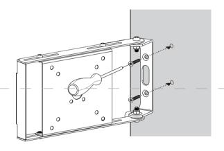
3. Fix it with screws on the wall.
