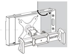
4. The bracket can adjust the angle, and it can also fit perfectly to the wall.
