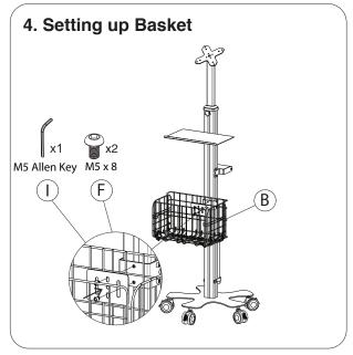
4A. Identify the metal plate around the center of the body. Align holes to the basket holes (B) as shown and rotate in screws (F) using provided tool (I) until securely tightened.
