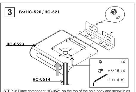
STEP 3: Place component HC-0521 on the top of the pole body and screw in as shown. Attach HC00523 and screw in. Attach storage tray afterwards with tools as shown.
