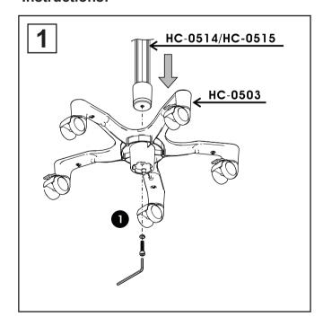
STEP 1: Place desired central pole body into the base and screw in the bolt/washer as shown with the included tools
