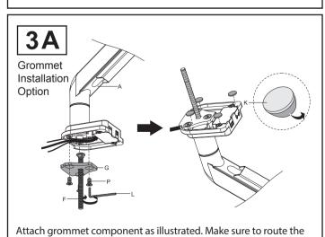
wires onto the exterior hook feature to neatly route the wires.
