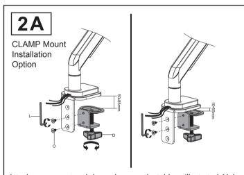
Attach component and clamp down on the table as illustrated. Make sure to route the wires onto the exterior hook feature to neatly route the wires as illustrated.
