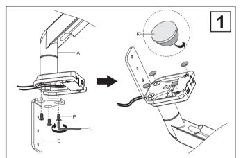
Setup mounting base as illustrated. Be sure to have all the wires pulled out before screwing on the mounting base.
