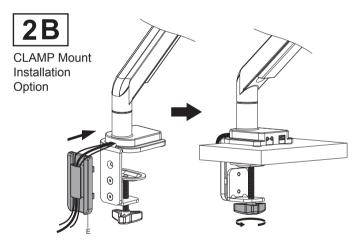
Attach component and clamp down on table as illustrated.
