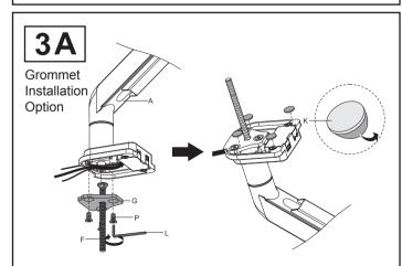
Attach grommet component as illustrated. Make sure to route the wires onto the exterior hook feature to neatly route the wires.
