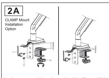
Attach component and clamp down on the table as illustrated. Make sure to route the wires onto the exterior hook feature to neatly route the wires as illustrated.
