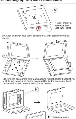
2C. If needed, lay-in correct included masking insert(H). Close and lock enclosure afterwards and you're set
