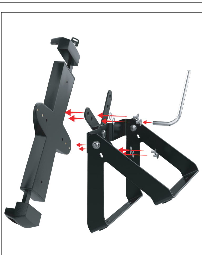
A. Install Holder to VESA. Screw in provided nails, washers and nuts as illustrated (Shown Above)
