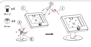
3A. Align enclosure (C) holes to VESA plate (A) holes. Turn in Screws M5 X6 (D) above using provide tool (J) while holding hex nut (E) From behind with fingers. Shown Above.
