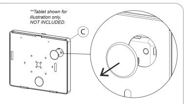
5A. When installing device into the enclosure, identify where the camera is. Then simply remove and pop out the cover prior to mounting or setting up tablet to properly expose camera.
