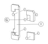
4A. Identify the double sided adhesives (G). Peel away the backing on both sides. Adhesive four of them behind the foam pieces (I) as illustrated. They are to adhese the foam to the enclosure. Peel away the back on the next four and place them on top of the foam pieces as illustrated. These are to attach the foam to the tablets and ensure security.
