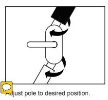
Push joint clasp back inward to lock joint in place.
