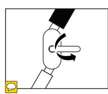
Lock the knob to tighten universal joint again.
