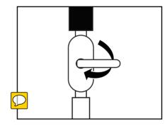
Release the knob to loosen the universal joint.
