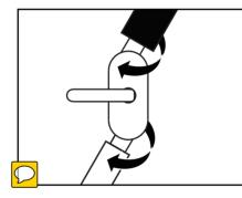
Adjust the pole by rotating the pole and universal joint.
