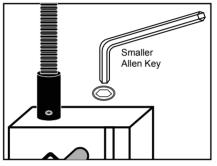
2. Use the smaller Allen key to screw up two meter screwes insde the gooseneck, tightening the connection.
