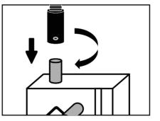
Screw gooseneck onto the male metal connection bolt on top of the clamp.
