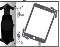
1. Press the button on the side of the holder center to slide out holder arm. Insert your tablet against the spring end, then slide the other arm back in, closing firmly.
