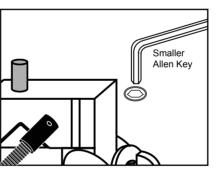
4. Use the smaller Allen key to screw the two meter screws insde the gooseneck, tightening the connection.
