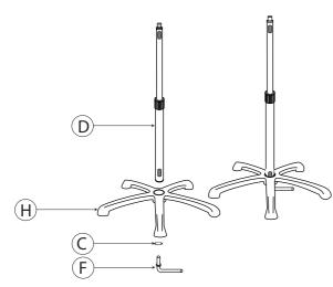
2A. Align the bottom of pole body (D) to the top center of the base (H). While pieces are connected, securely flip over so you can see the bottom. Align washer (C) to the hole on the bottom. Using your hands, identify L-shaped component (F) and rotate through the washer into the hole until securely tightened. Pole body and base should now be securely attached to each
