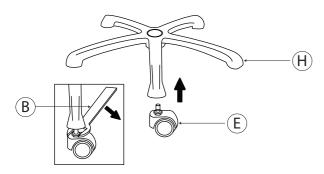
1A. Take one wheel (E) and align it to the leg arm holes on the underneath of the base (H). Initially you can use your hands and manually rotate the wheel until slightly tightened. Then use the provided wrench tool (B) at the hex shaped area and rotate it securely to tighten the rest of the way.
