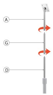
4A. First add the body extension pole (G) Connect the male to female adapters and rotate until securely attached. Afterwards, repeat the same exact process for VESA add-on component.
