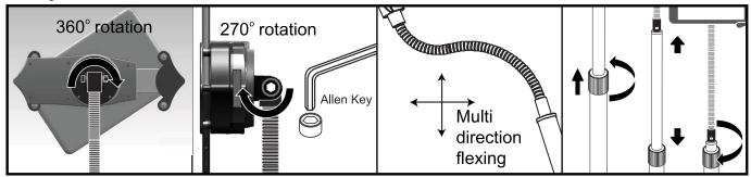
Use the bigger Allen key to tighten and loosen the gooseneck connection screw, adjusting ease of rotation in the tablet holder.
