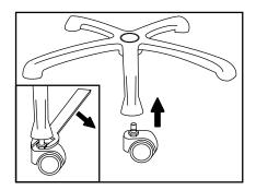
Screw wheels into floor base by hand, then use wrench to tighten.
