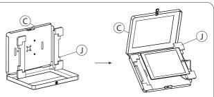
3B. Find the appropriate size foam padding (J) for the tablet you wish to use. Make sure device is compatible for the enclosure (C). Lay in device and connect any cables/cords as needed.
