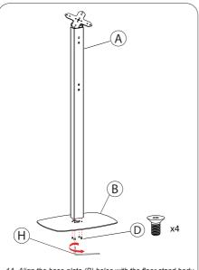
1A. Align the base plate (B) holes with the floor stand body (A) and rotate in screws (D) using the provided allen key (J) until securely tightened.
