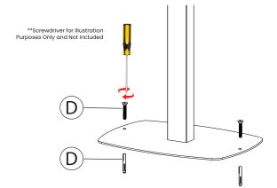
10A. Using a power drill or similar (note provided) that is the same size as your metal anchor - create a cavity in the floor. Insert the base part of the metal anchor (D), and screw in the nail component of the metal anchor (D) from above with a screwdriver (not provided) until securely tightened. Repeat for all holes.
