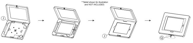
6A. Insert the appropriate foam piece (J) that is compatible with your tablet.
