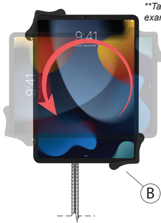
5A. For landscape or portrait setups, rotate the holder (B) as shown above.
